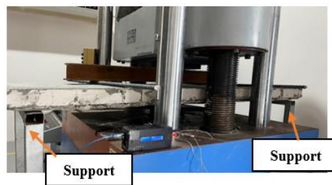
Figure 4. The method for testing the bending strength of the wall
